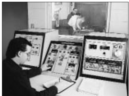
Dynamometer testing is required to determine accurate motor efficiencies.
