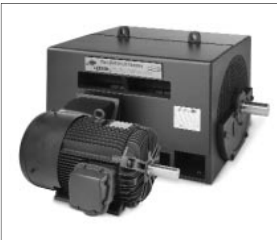
Two types of industrial motors: the ribbed frame version in the foreground is a good example of a NEMA T frame motor covered under EPACT through 200 HP. The larger motor is “above” NEMA frame size; therefore, it is exempt from EPACT mandates as now written.
